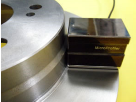
MiniProfiler: roughness measurement of brake discs
